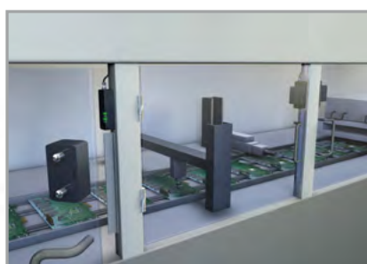
Door guarding on pick and place machine
