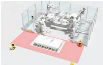
Safety solutions, e.g. for safe guarding transfer stations and access guarding at transport systems
