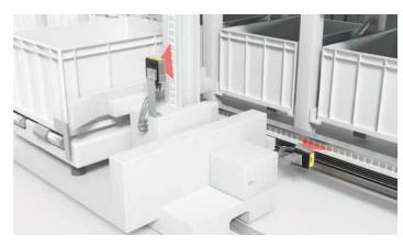
The FBPS 600i is particularly suitable for position detection during fast movements, such as for use on rack and conveyor systems. The FBPS 600i has a very short error response time of only 10 ms. This allows speed curves and handling performance to be optimized.
