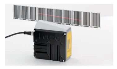
The FBPS 600i operates with exceptional reliability. Each scanning process reads multiple codes, from which the software determines highly accurate position values. The oblique path of the scanning beam and the movement of the device ensure that each code is scanned at different points. This prevents reading errors caused by local contamination or damage.
