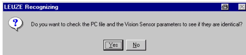
Selecting comparison starts the same procedure as described in comparison of versions. Then loading and transmitting of data to the sensor starts. The progress indicator provides you with information on the transmission status. After ending the display vanishes, and you can work on with new data.
