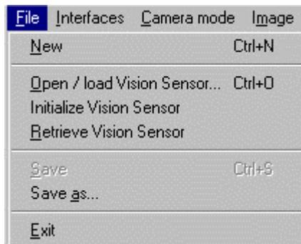
This loads the file into the program and passes it on to the vision sensor via serial interface. If the last changes of your current file were not saved, you receive a corresponding message.
