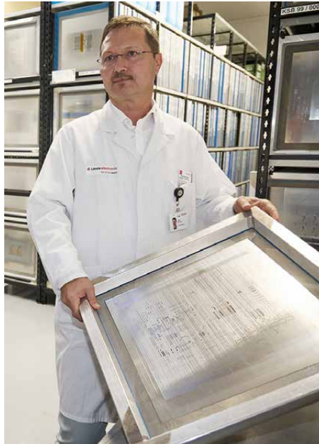
Production Manager Georg Denking with a stencil. It is used to apply the solder paste specifically to the circuit boards.
