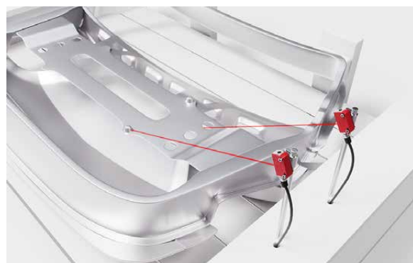
Our ODT3CL1-2M laser light scanners can not only detect the presence of the component but also defined reference points on a component, thus controlling quality. The sensors also work reliably with different surface finishes.
