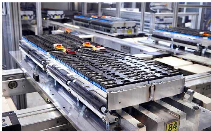
A double module including cell contact system on the upper side. In the last step, a cooling unit is added. The double module then goes to the assembly area. Leuze sensors detect the position of the modules on the conveyor belt.
