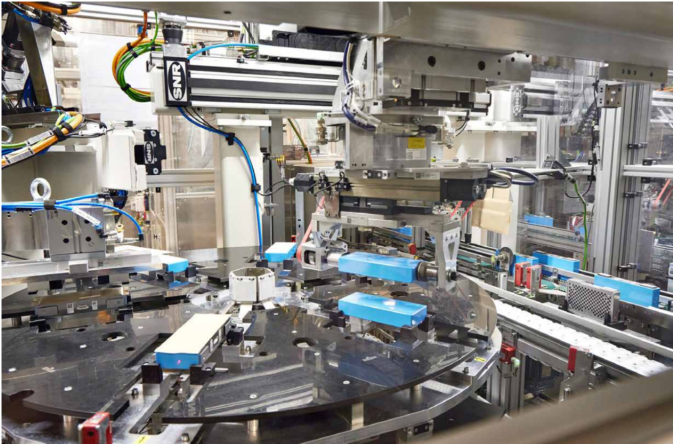
At this station, each cell receives a “heat shield”—a protective heat insulation—which is pressed onto the longitudinal sides. Leuze PRK 25 reflection light barriers detect the presence of the objects.
