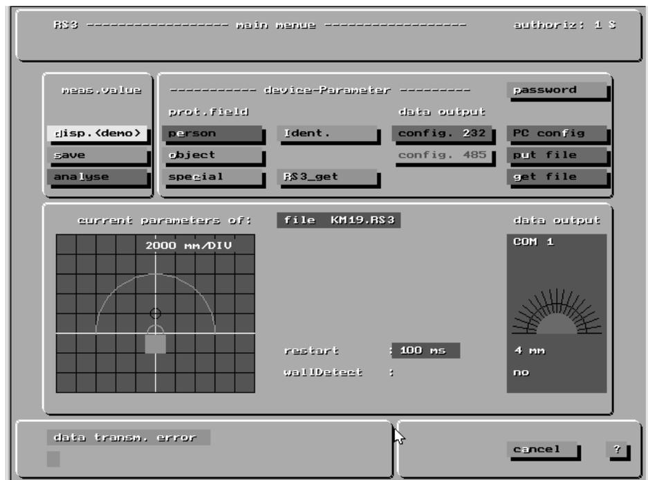
**Measurement value** Opens the window "Settings" for configuring the contour display. Continuing with the window "Display", the current distance measurement data are displayed as a 2D-contour and the status of the protection field is indicated.
