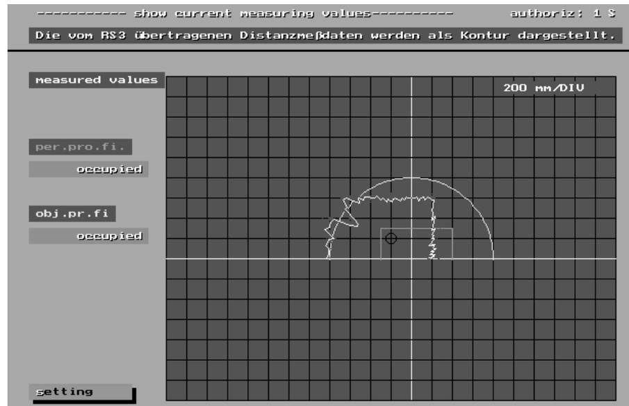
The status of the superimposed protection field is displayed in the top left-hand area of the window.
