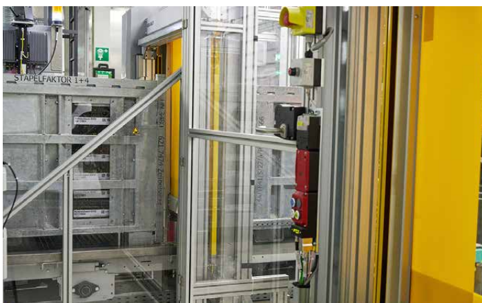
To ensure that the large load carriers (GLT) can be safely loaded and unloaded, a Leuze MLC series safety light curtain protects the hazardous area against access by persons. Muting ensures that only the LLC can pass.
