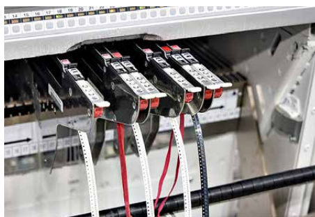
The standard electronic components are located on rolls. The individual conveyor belts are fed into a placement machine. This places the components on the printed circuit board.
