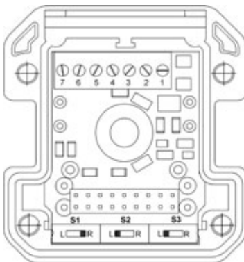
Fig. 8.2-1: Transmitter connection cap, switch positions
