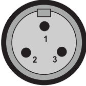
Fig. 7.4-1: Plug, MIN-series 3-pin – view of the plug pins of the transmitter
