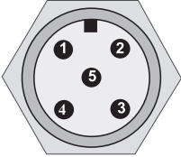
Fig. 7.8-3: Receiver machine interface /A1, M12 5-pin device plug (view of the pins)
