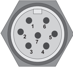
Fig. 7.4-2: Receiver/transceiver machine interface /T3, MIN-series (view of the pins)
