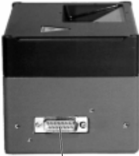
15 pin SubD type connector (male)
