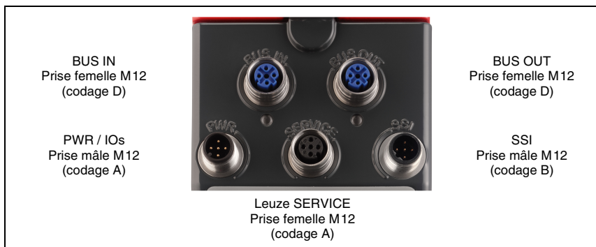
Figure 7.1 : Raccordements de l'AMS 348i SSI
