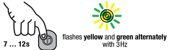
Adjusting the switching behavior of the switching output – light/dark switching
