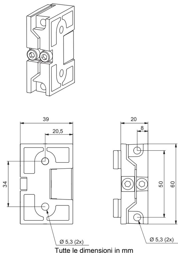
Figura 15.6: Supporti orientabili BT-2SB10/BT-2SB10-S
