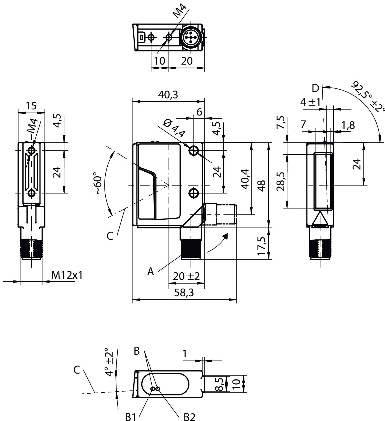
A Turning connector, turnable by 90°
