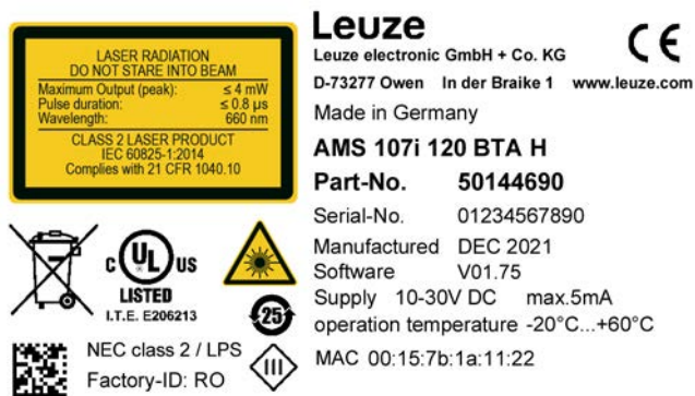
Fig. 5.1: Name plate of AMS 107i
