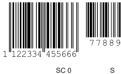
Fig. 16.8: Code type: EAN 13 add-on
