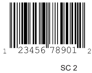
Fig. 16.6: Code type: UPC-A
