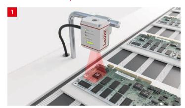
**Solution:** The DCR 100i code reader features DPM decoding and a manually adjustable focus, enabling reliable capture of small codes.
