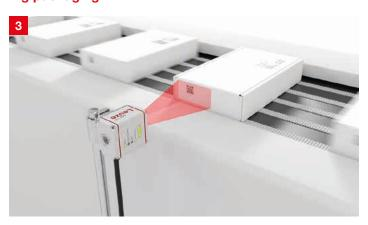
Solution: The DCR 100i features an imager that captures 120 images per second (for conveyor speeds up to 2 m/s) and includes powerful integrated illumination. It captures bar codes on moving objects quickly and accurately, reduces reading errors and increases throughput in demanding applications.
