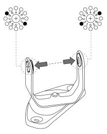
4. Insert the sensor and the tamper-proof screws in the bracket (see How to insert the sensor on the next page).
