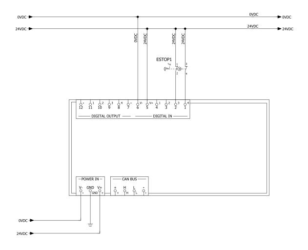
Note: the indicated emergency button opens the contact when pressed.
