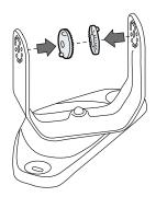
3. Reinsert the adjustment ring in the bracket holes according to the unit value of the desired inclination degrees (see How to choose the adjustment ring position on the next page).
