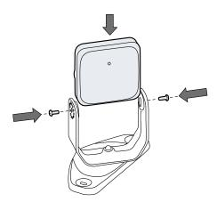
5. Tilt the sensor downward or upward the number of notches corresponding to the tens place value of the desired angle (for example, for an inclination angle of +38°, the tens place value is 3: tilt the sensor upward three notches).
