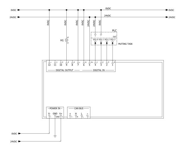
Note: the cables used for wiring the digital inputs must have a maximum length of 30 m (98.4 ft).
