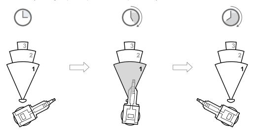
In this case, it is possible to ignore the detection signal in the detection field 1, thus avoiding unnecessary downtime.
