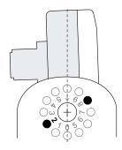
3. Tilt the sensor upward of six notches.
