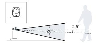
Side view with sensor inclination 0°.
