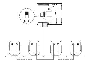
Chain with controller inside the chain and two sensors with bus terminator
