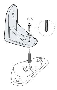
3. Mount the bracket with the sensor and the aligning ring. Use the tamper-proof screw provided with the bracket.
