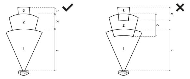
The detection distance of one or more fields can be 0 (e.g., detection field 3). The first detection field with a detection distance other than 0 (e.g., detection field 1) must have a minimum detection distance of 200 mm.
