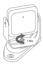
5. Loosen the tamper-proof screws to tilt the sensor.
