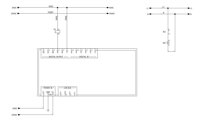
Note: the cables used for wiring the digital inputs must have a maximum length of 30 m (98.4 ft).
