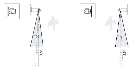
Top view with sensor inclination 0°.
