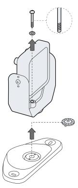
2. Attach the roll bracket to the base. Use the tamper-proof screw provided with the bracket.
