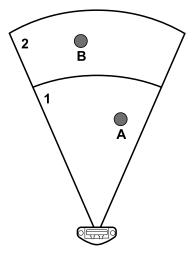
In this example, detection field 1 generates a detection signal for target **[A]** but target **[B]** could not be detected.
