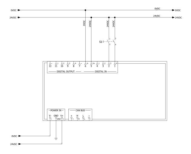
Note: the button indicated for the restart signal closes the contact when pressed.
