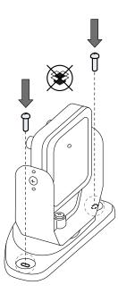
2. With an Allen key, loosen the screw at the bottom to pan the sensor.
