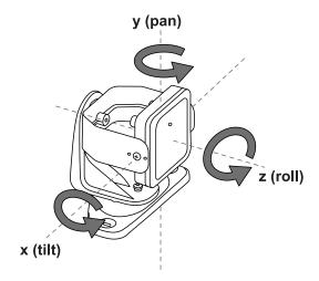
When the system configuration is saved, the sensor also saves its position. Later, if the sensor detects changes in rotation around these axes, it sends a tamper alert to the controller. Upon reception of a tampering signal, the controller deactivates the safety outputs.
