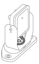
3. Pan the sensor until it reaches the desired position.
