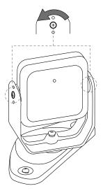
6. Tilt the sensor to the desired inclination (see Sensor position on page 76).
