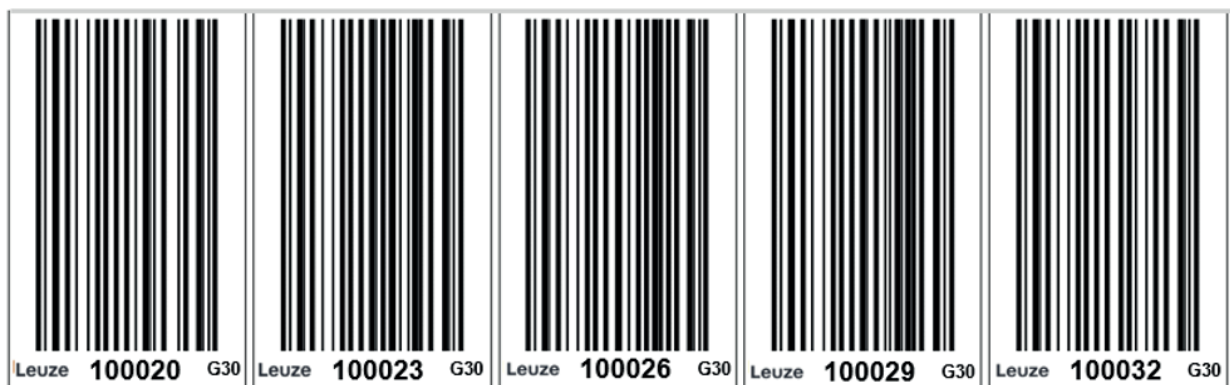
Fig. 4.2: Example BCB G30 bar code tape, beginning with position value 1000.20 m, ascending in increments of 3 cm
