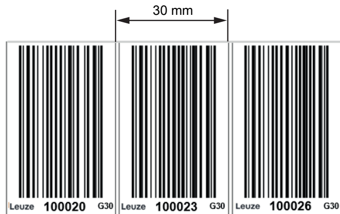
Fig. 6.11: Example: Checking the dimension of 30 mm on the self-printed online repair bar code tape
