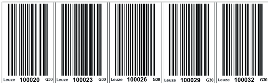
Fig. 6.1: G30 bar code tape, beginning with position value 1000.20 m, ascending in increments of 3 cm / 30 mm. Lined up sequentially without interruption, the bar codes produce a digitized tape measure with a grid of 30 mm or 40 mm.
