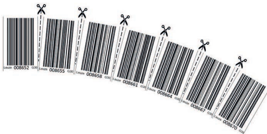
Fig. 6.9: Preparing the bar code tape for use in vertical curves
