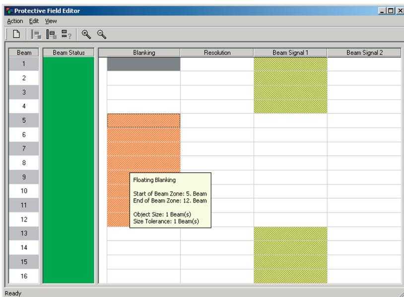
Bild 12.1-1: Parameterization of protective field for sample application punch machine
