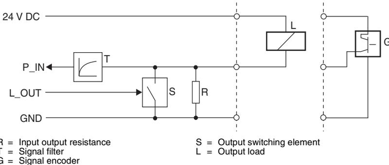
**Bild 5.3-5:** Layout of inverse inputs/outputs – working principle
