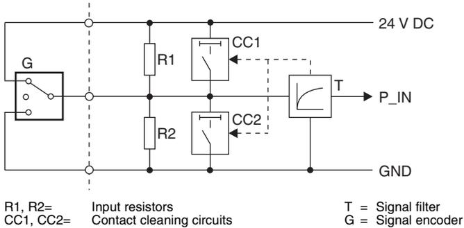
**Bild 5.3-3:** Layout of tristate inputs – working principle
