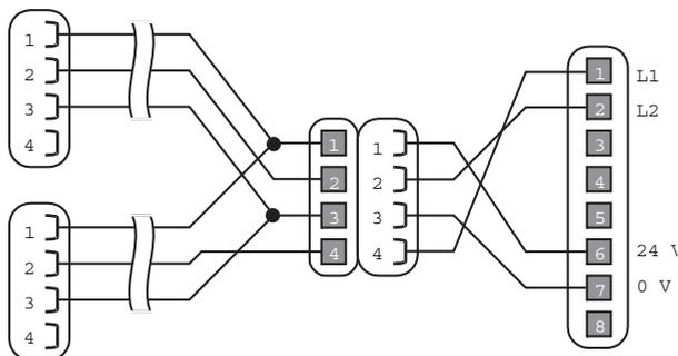
**Bild 11.2-4:** Layout of cable splitter AC-SCC2
