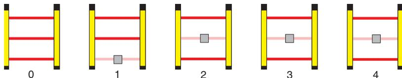
**Bild 7.7-2:** Beam-related multiple scanning, scan number 3 (example)
