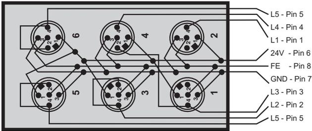
**Bild 11.2-2:** Internal wiring of the local connection box
