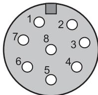
**Bild 11.2-1:** Receiver/transceiver – local socket M12, 8-pin
