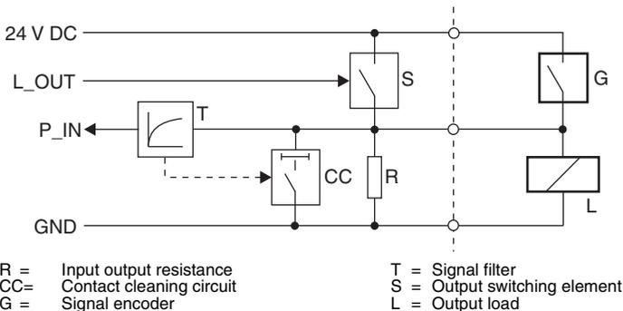
**Bild 5.3-4:** Layout of standard inputs/outputs – working principle
