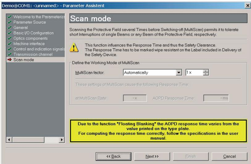
**Bild 7.7-4:** "MultiScan" window with floating blanking in the protective field
