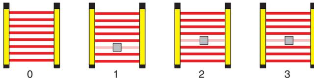
**Bild 7.7-1:** Scan-related multiple scanning, scan number 3 (example)
