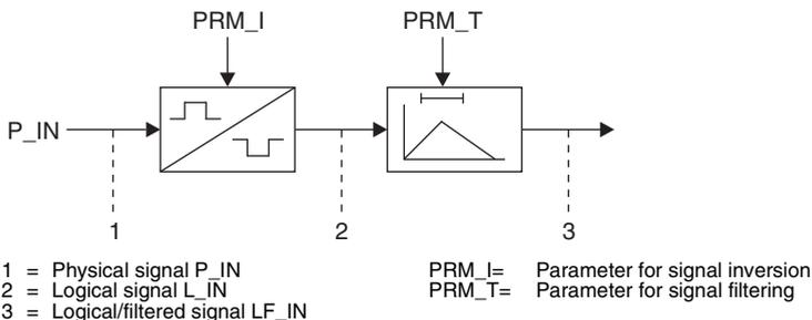
**Bild 5.3-6:** Layout of control signal processing chain – working principle
