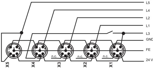
**Bild 11.2-3:** Internal wiring of the local connection field
