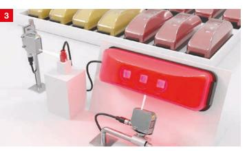
**Solution:** In the first process step, a CRT 648 color sensor checks the color of the connector. Another CRT 648 checks whether the rear light has the correct light color and intensity.
