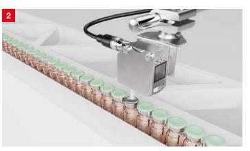
**Solution:** The CRT 648 color sensors with luster suppression detect the high-gloss vial caps while ensuring process stability. Operating and adjusting the sensors is quick and easy thanks to the large LC display.
