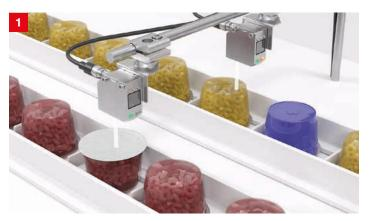
**Solution:** The new CRT 648 color sensors can be taught up to seven colors. They are equipped with a large light spot and reliably detect the colors of both the packaging and the cover. The large operating range of up to 150 mm ensures reliable detection, even when switching to other formats.
