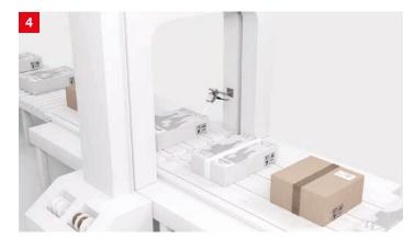
**Solution:** The CRT 648 series color sensors detect the carton color and transmit the information to the strapping machine. This allows the system to select the appropriate strap color.
