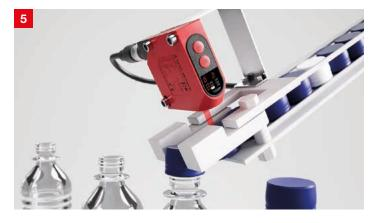
**Solution:** The taught color of the cover is detected by the CRT 448 and incorrect covers are sorted out by the output signal of the sensor with sorting device.
