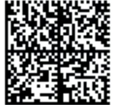
Scanning the adjacent 2D-code sets the following interface parameters for keyboard emulation via USB interface:
