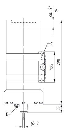
A Reference edge for the measurement (distance zero
