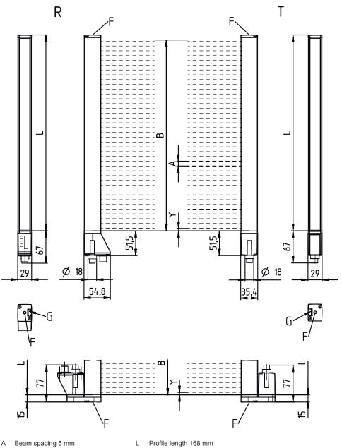
A Beam spacing 5 mmB Measurement field length 160 mm
