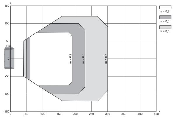
Х Reading field distance [mm]
