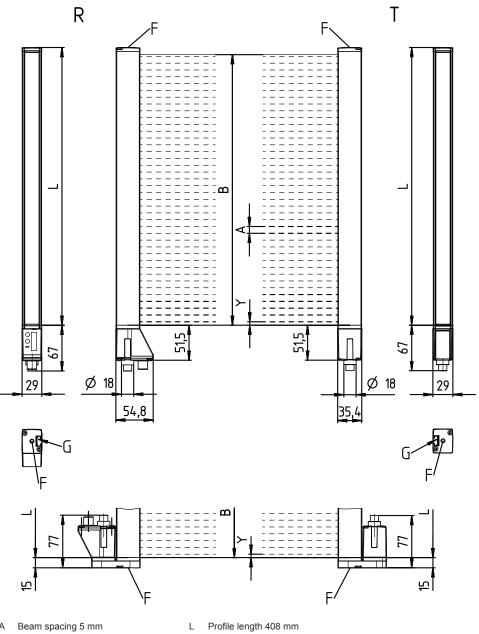
Beam spacing 5 mm А В Measurement field length 400 mm
