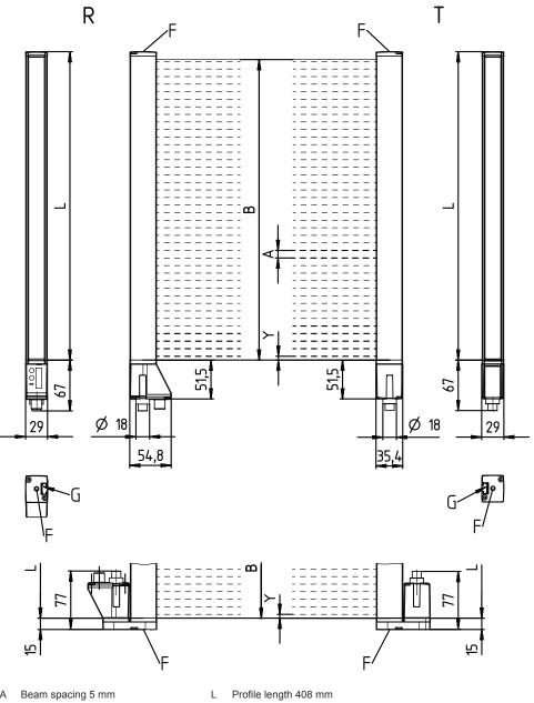
Beam spacing 5 mm А В Measurement field length 400 mm
