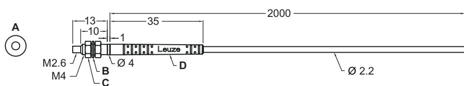
A Ø 1.0 mm plastic fiber core x 1 pc      D Bend protection, PVC
