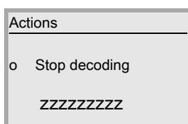
Once the bar code is detected, the laser beam is switched off again. The read result **zzzzzzzz** is shown directly in the display for about 1 s. After that, the Actions menu is displayed again.
