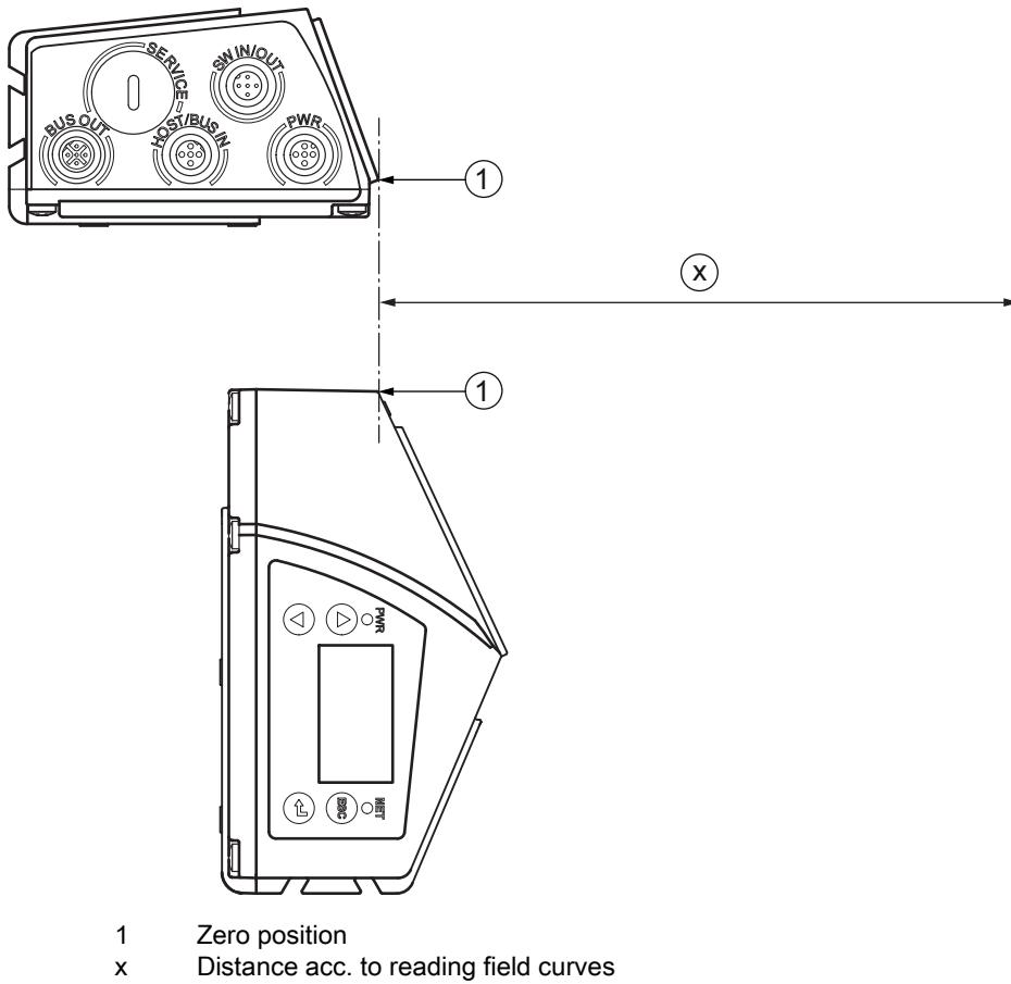
Figure 15.7: Zero position of the reading distance
