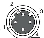
Figure 7.10: Host/BUS IN, M12 socket (D-coded)
