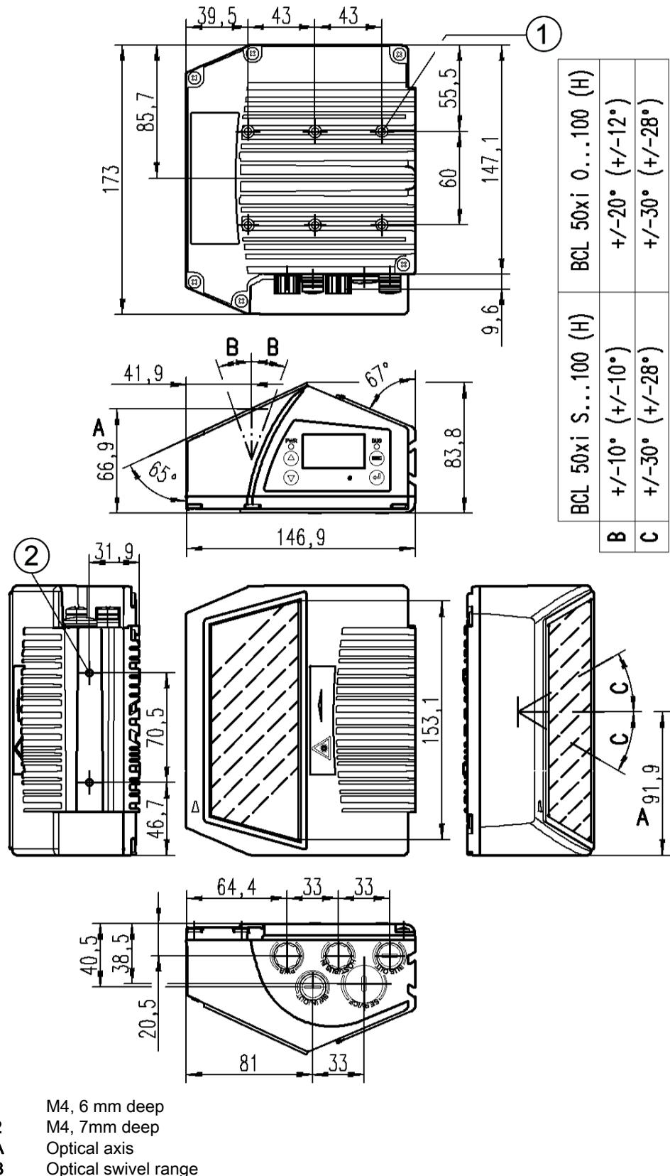
Figure 15.2: Dimensioned drawing of oscillating-mirror scanner
