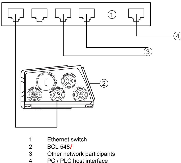
Figure 7.13: PROFINET-IO in a star topology
