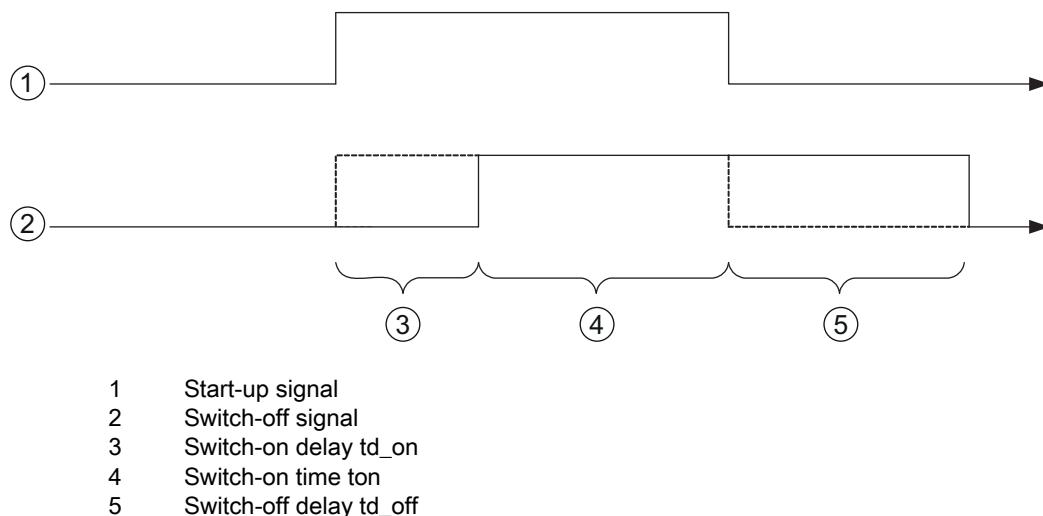
Figure 10.8: Switch-on delay in input mode
