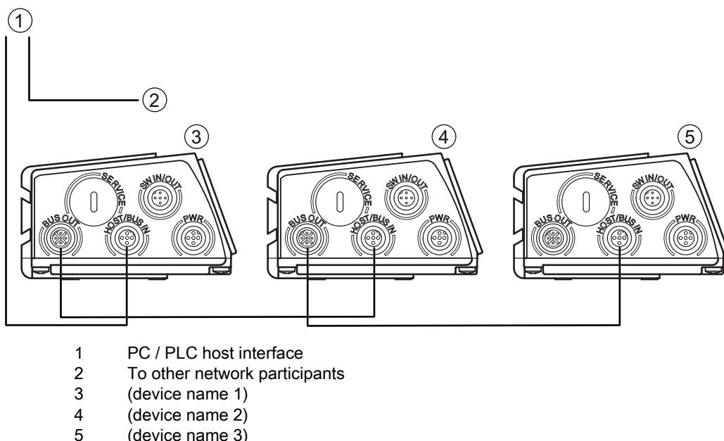
Figure 7.14: PROFINET-IO in a line topology
