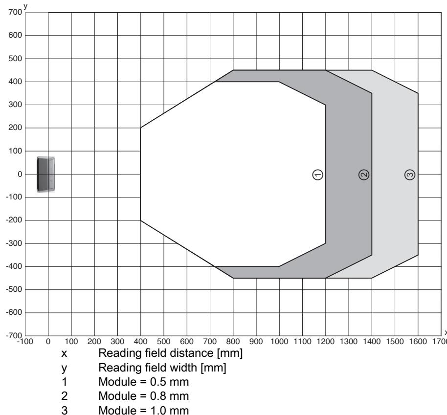
Figure 15.27: "Low Density" reading field curve for oscillating-mirror scanners with heating
