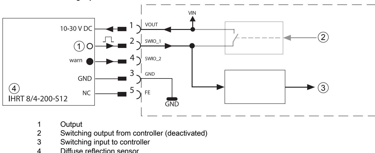
Figure 7.8: Switching input connection diagram SWIO\_1 and SWIO\_2
