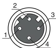
Figure 7.12: M12 socket (D-coded)
