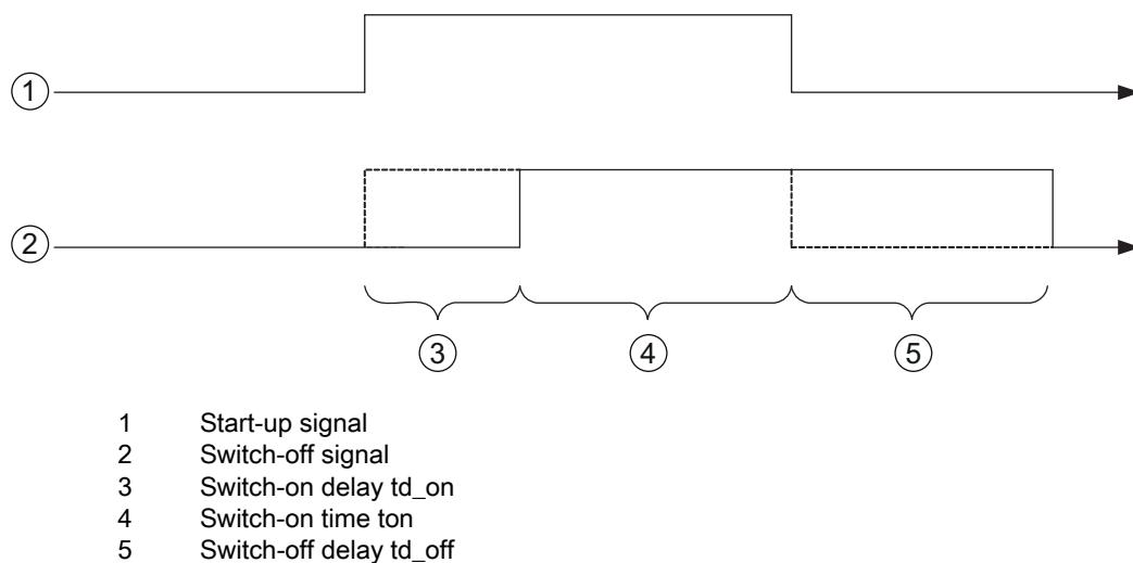
Figure 10.9: Switch-on time in input mode
