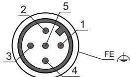
Figure 7.3: PWR, M12 connector (A-coded)
