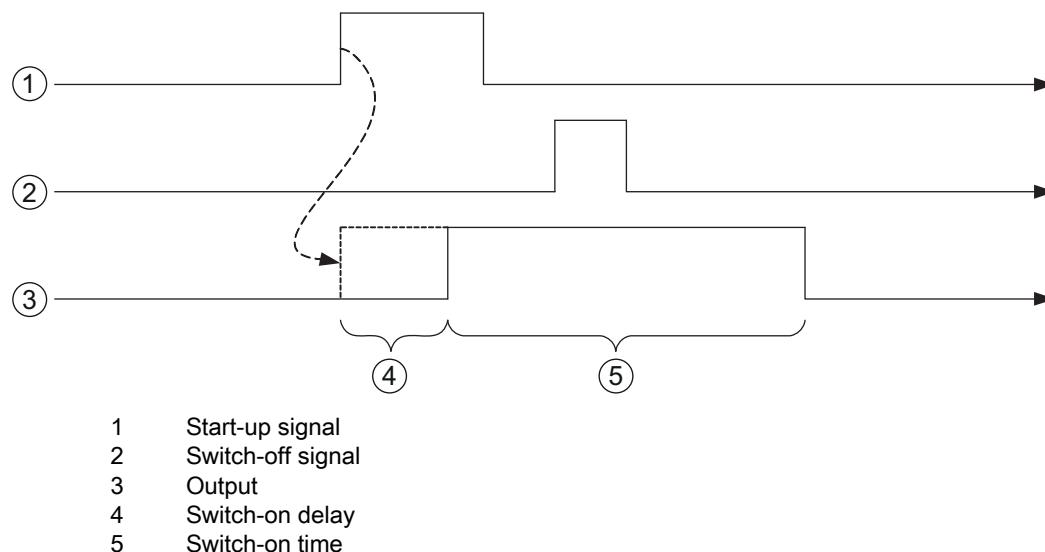
Figure 10.6: Example 2: Switch-on delay > 0 and switch-on time > 0
