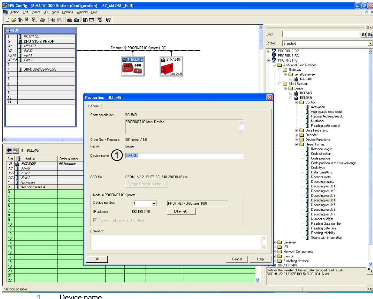
Figure 10.1: Assignment of the device names to IP addresses
