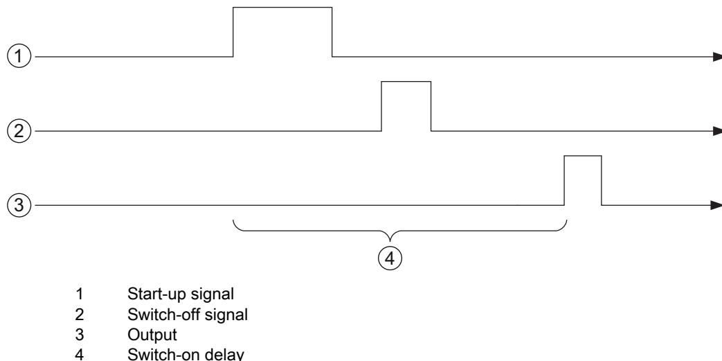
Figure 10.7: Example 3: Switch-on delay > 0 Switch-off signal prior to lapsing of the switch-on delay
