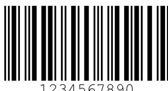
Figure 17.9: Code type 01: Interleaved 2 of 5
