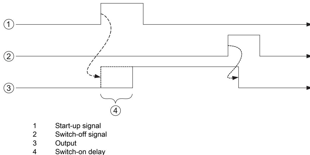
Figure 10.5: Example 1: Switch-on delay > 0 and switch-on time = 0
