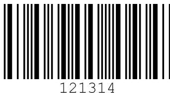
Figure 17.15: Code type 11: Codabar
