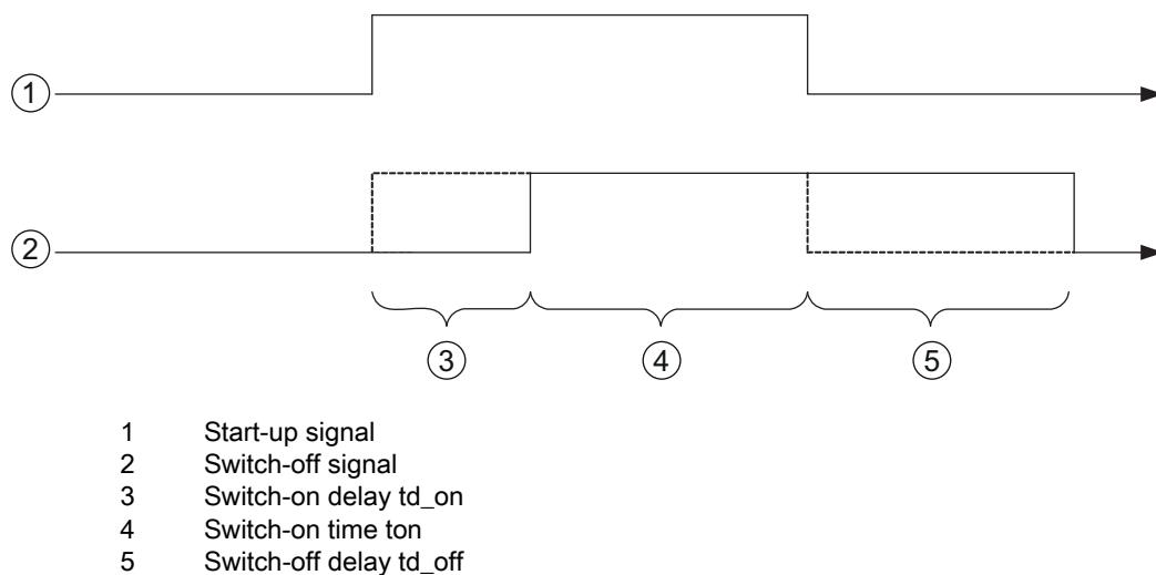
Figure 10.10: Switch-off delay in input mode
