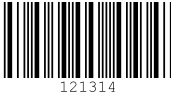
Figure 16.15: Code type 11: Codabar
