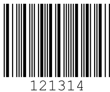
Figure 16.7: Code type 11: Codabar
