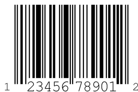
Figure 16.3: Code type 06: UPC-A
