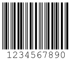
Figure 16.1: Code type 01: Interleaved 2 of 5
