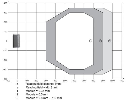
Figure 15.12: "Medium Density" reading field curve for oscillating-mirror scanners
