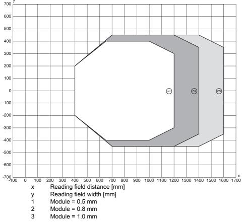
Figure 15.26: "Low Density" reading field curve for line scanner with heating The reading field curves apply for the reading conditions stated in Table 15.5.
