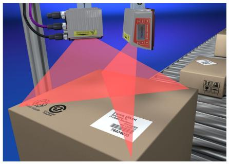
Figure 5.3: Principle arrangement for omnidirectional reading
