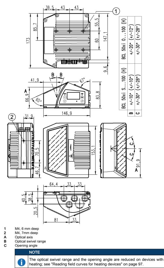
Figure 15.2: Dimensioned drawing of oscillating-mirror scanner
