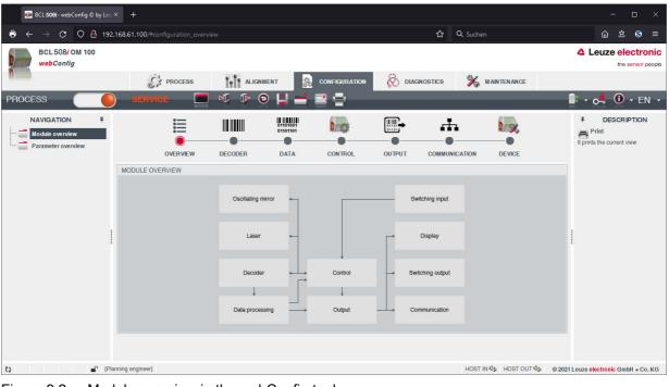
Figure 9.2: Module overview in the webConfig tool
