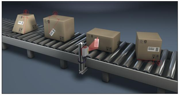
Figure 4.1: Possible bar code orientation
