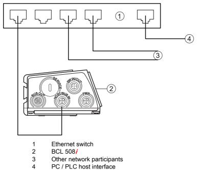
Figure 7.13: Ethernet in a star topology
