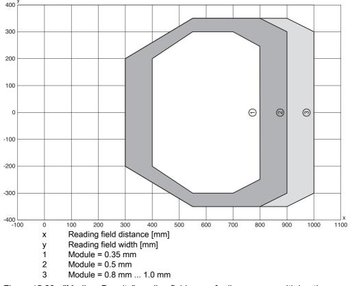
Figure 15.23: "Medium Density" reading field curve for line scanner with heating The reading field curves apply for the reading conditions stated in Table 15.5.
