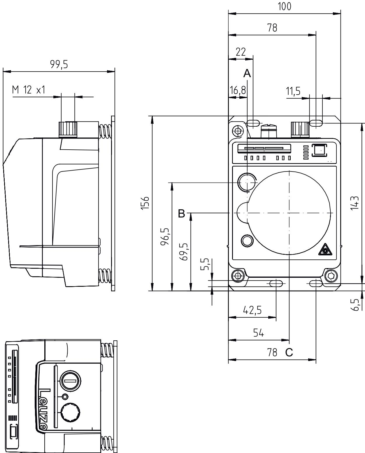
A Center axis of transmitter and alignment laser
