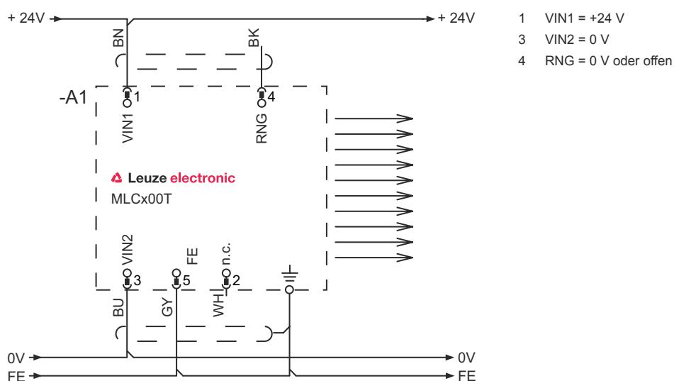
**Schaltbilder****Übertragungskanal C1, Standard-Reichweite**
