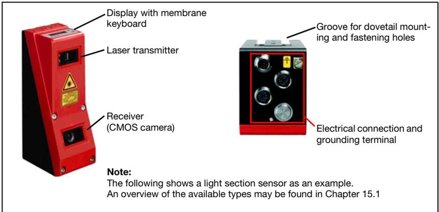
Figure 4.1: Mechanical design of Leuze light section sensors
