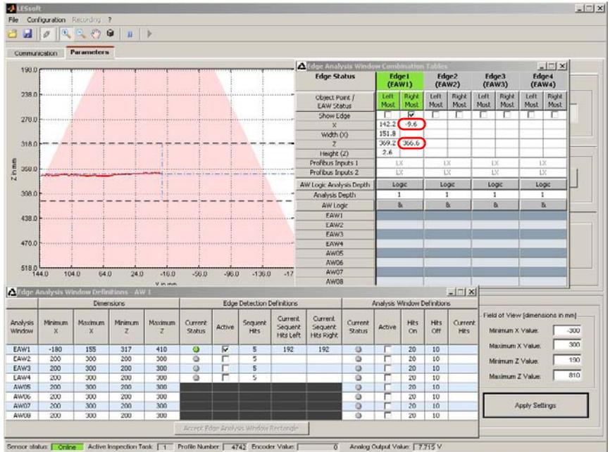
Figure 9.7: Application example 1: web edge measurement
