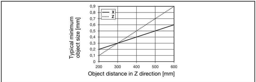
Figure 3.4: Typical minimum object size LES 36HI...
