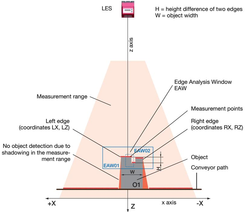
Figure 4.9: Edge detection with varying object position
