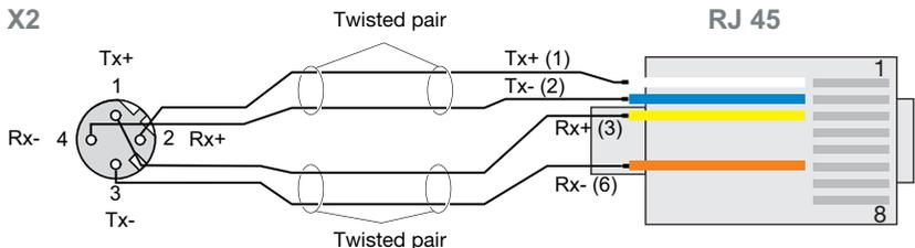
Figure 6.7: HOST / BUS IN cable assignments on RJ-45
