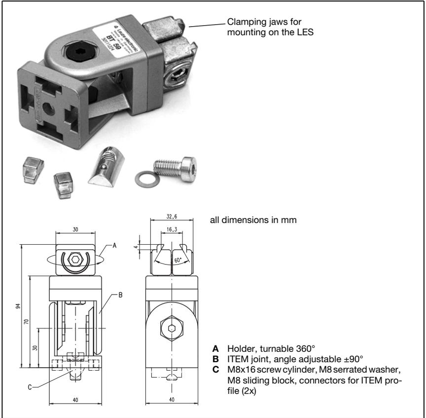
Figure 5.5: BT 59 mounting device
