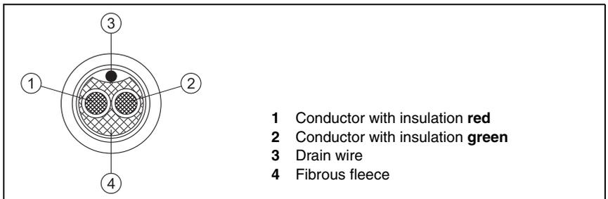
Figure 15.1: Cable structure for PROFIBUS connection cable
