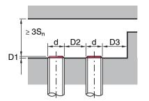
S<sub>n</sub> [mm] 22 D1 [mm] 6 D2 [mm] 110 D3 [mm] 30
