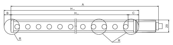
$H_{\mathrm{PFE}}$  Effective protective field height = 1678 mm H<sub>PFN</sub> Nominal protective field height = 1650 mm
