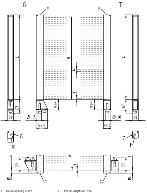
Beam spacing 5 mm А В Measurement field length 320 mm
