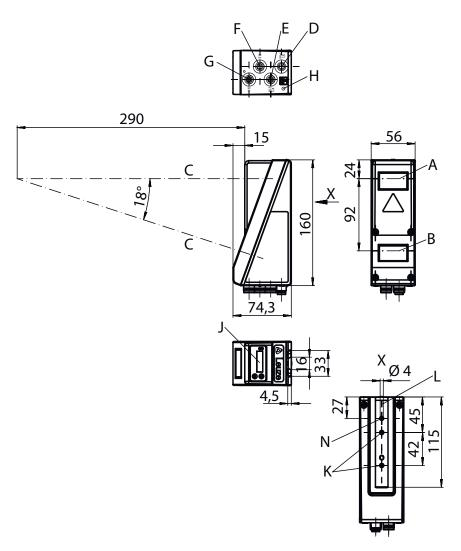
Transmitter В Receiver С Optical axis D, E, F, G X1-X4 connections
