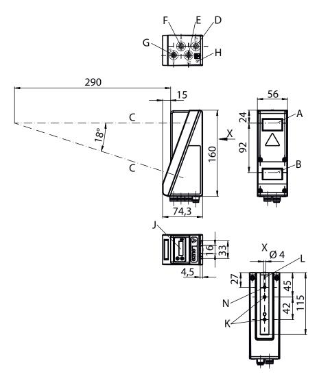
Transmitter В Receiver С Optical axis D, E, F, G X1-X4 connections Н FE screw
