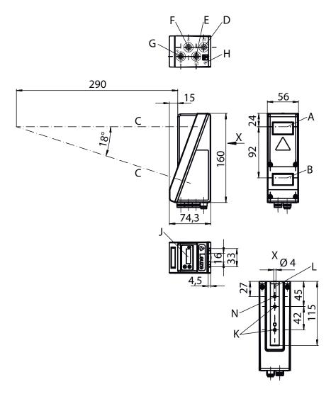
Transmitter Receiver Optical axis D, E, F, G X1-X4 connections
