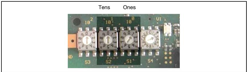
Figure 3.2: Rotary switch for setting the address
