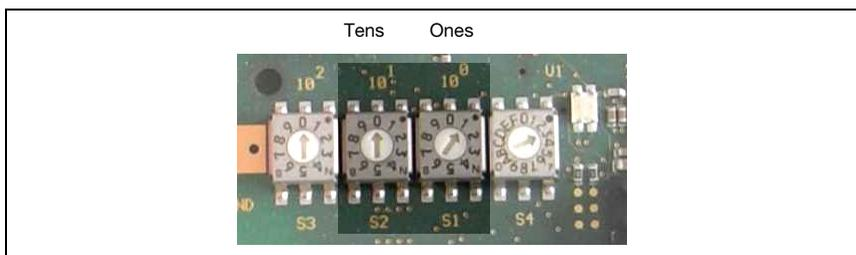
Figure 12.1: Rotary switch for setting the address
