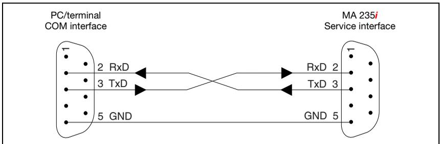
Figure 7.6: Connecting the service interface to a PC/terminal
