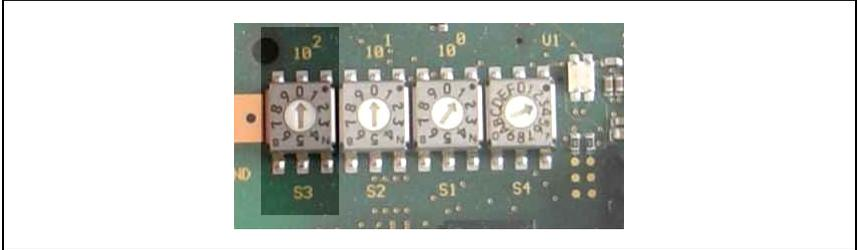
Figure 12.2: Rotary switch for setting baud rate
