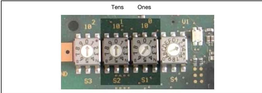
Figure 8.6: Rotary switch for setting the address
