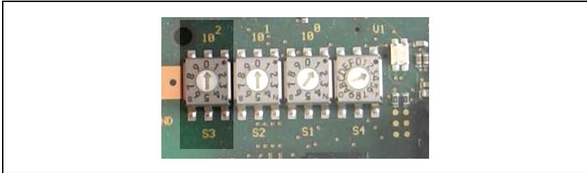
Figure 3.3: Rotary switch for setting baud rate
