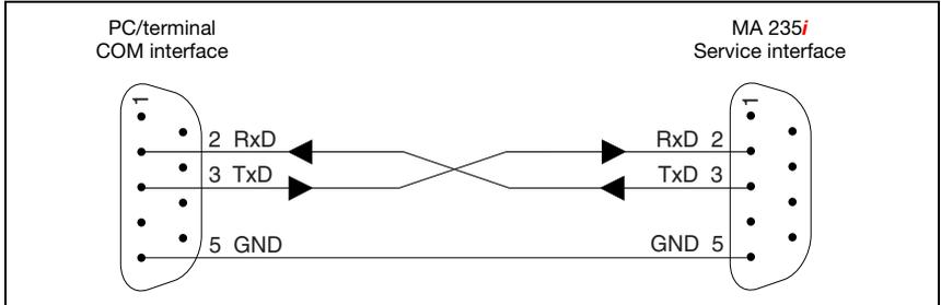
Figure 4.3: Connecting the service interface to a PC/terminal
