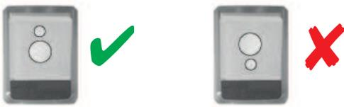
Fig. 6.28: Orientation of the diffuser foil
