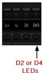
1. Insert the IO-Link device negative wire into the **L-** contact and tighten the wire-clamp screws to prevent the wire from coming loose.
