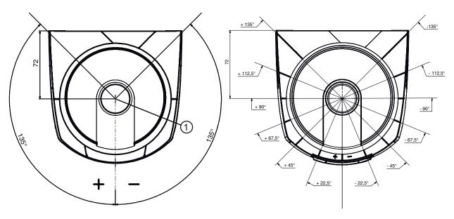
Reference point for distance measurement and protective field radius
