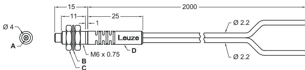
A Ø 1.0 mm plastic fiber core x 2 pc      D Bend protection, PVC
