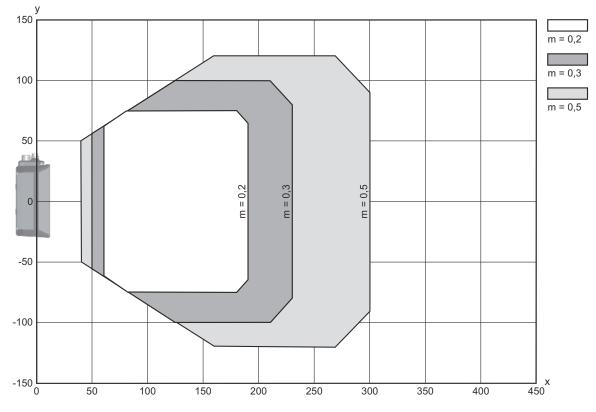
Х Reading field distance [mm]
