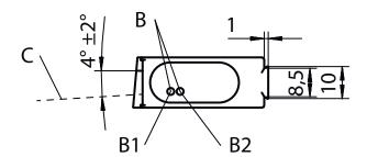
Turning connector, turnable by  $90^\circ$ А
