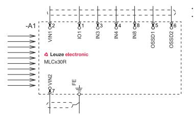
VIN1 = +24 V, VIN2 = 0 V: transmission channel C1
