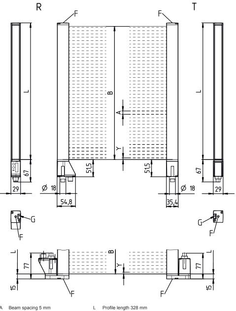
Beam spacing 5 mm А В Measurement field length 320 mm
