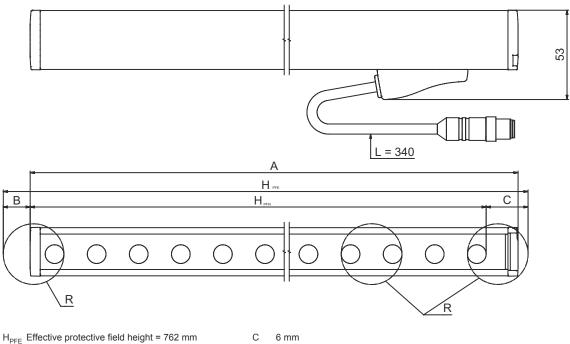
H<sub>PFN</sub> Nominal protective field height = 750 mm
