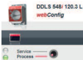
Fig. 9.4: Changing the operating mode (Process - Service)
